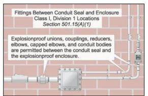
Electrical "Y-Seal", (EYS) prevent explosions from spreading through conduit systems and igniting outside atmospheres. When properly installed and filled with a ULlisted sealing compound, they create a physical barrier that minimizes passage of explosions from traveling freely through the conduit.
